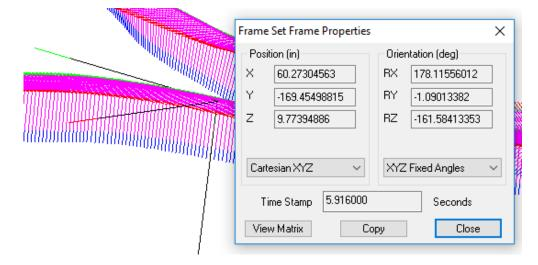
This provides access to both the transform and time stamp for individual frames. The time stamp is the super accurate controller time from the start of the scan.
