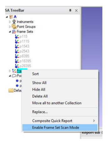
Once enabled, measurements are recorded graphically and can be accessed directly like a vector by double left-clicking on the frame of interest.
